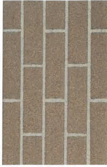
BRICK - VENEER SECONDARY (BR-B) MANUFACTURER: CUNNINGHAM BRICK SIZE: MODULAR - 3-5/8" x 2-1/4" x 7-5/8" MODEL: TAN VELOUR COLOR: (TAN) MORTAR: MATCH EXISTING - HOLCIM, DESERT BUFF
